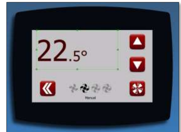
Using the SubscriptDigits property on a temperature display
